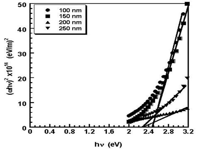
Fig.-3: Plot of  $(\alpha h\nu)^2$  vs.  $h\nu$  for ZnTe/Al films of different thicknesses.
