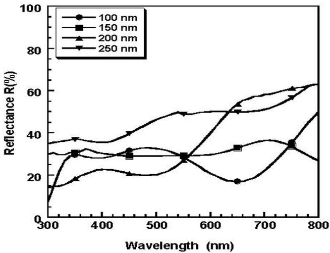
Fig. 2 Reflectance spectra of annealed ZnTe/Al thin films for 100, 150, 200 and 250 nm thicknesses.
