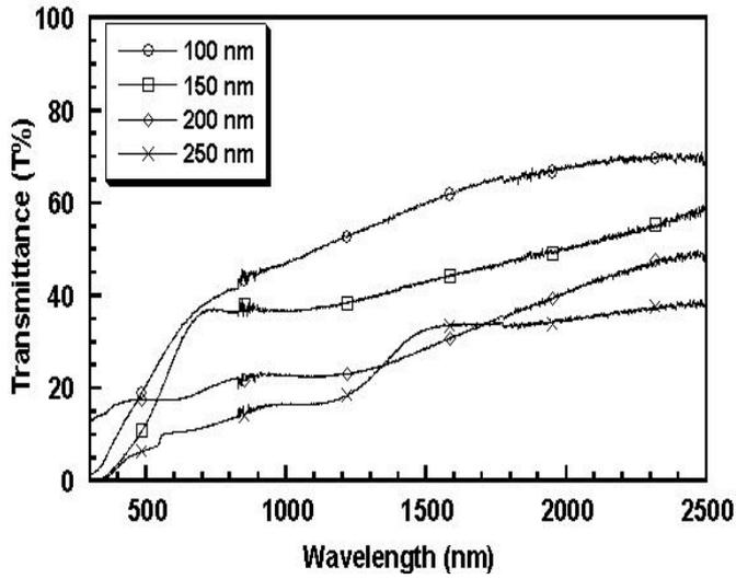
Fig. 1 Transmittance spectra of annealed ZnTe/Al thin films for 100, 150, 200 and 250 nm thicknesses.
