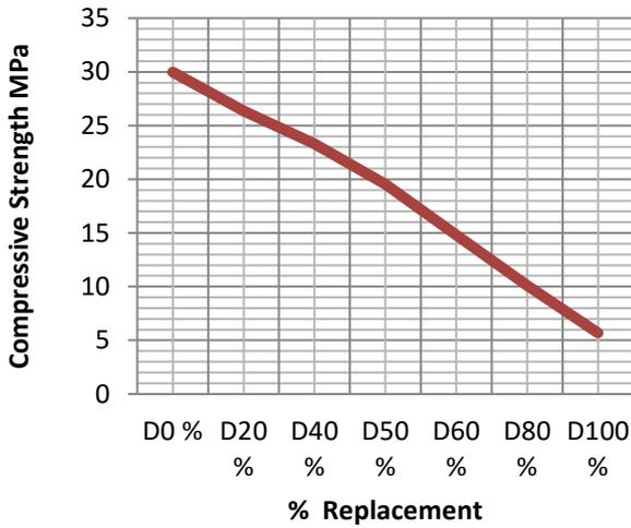
Fig. 8 Graph b/w % Replacement and compressive strength @ 7days
