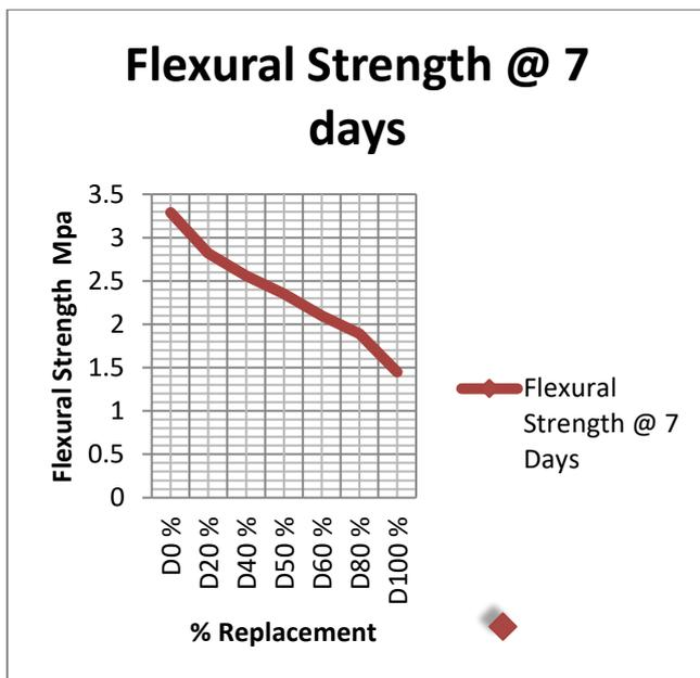
Fig. 11 Graph b/w % Replacement and Flexural strength @ 7days
