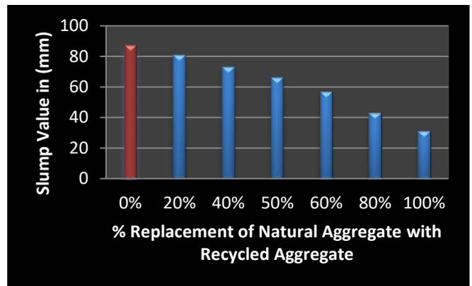
Fig. 5 Graph for Slump value at different % replacement of RA with NA
