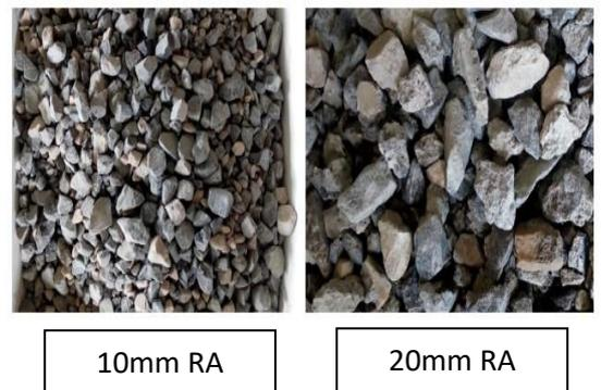
Fig. 4 Recycled Aggregate extracted in nominal size
