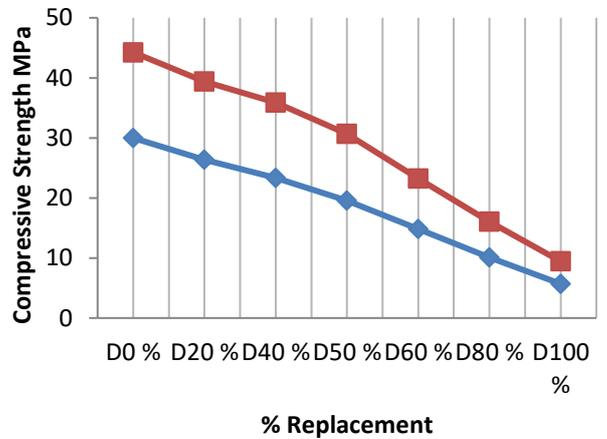
Fig. 10 Graph b/w % Replacement and compressive strength @ 7days and 28 days
