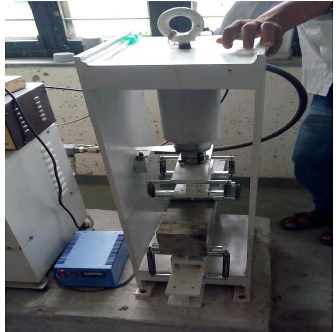
Fig. 7 Flexural strength testing machine
