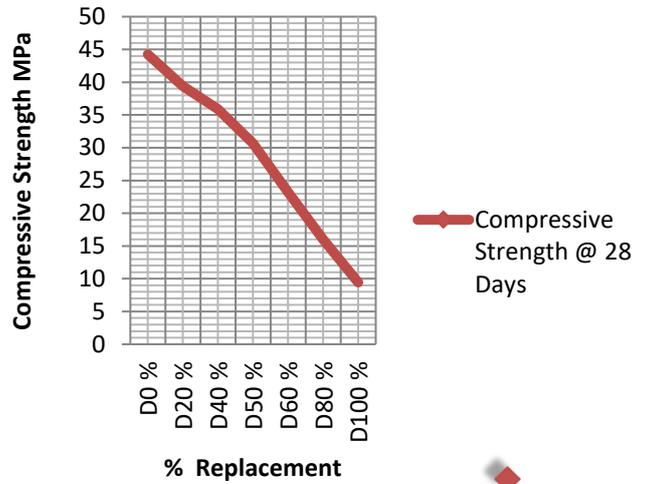
Fig. 9 Graph b/w % Replacement and compressive strength @ 28days
