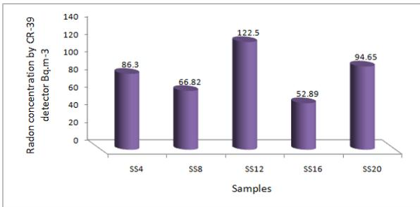
Fig.6 the radon concentrations measured by the CR-39 detector and samples to a depth of 60cm.
