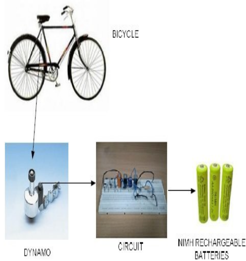
Fig.1 Charging batteries using bicycle pedal
