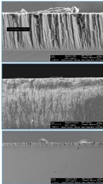
Fig.6. SEM image (cross-section) of porous silicon sample prepared by etching time 10 min at magnification (a)11450x, (b) 13650, (c) 1170x
