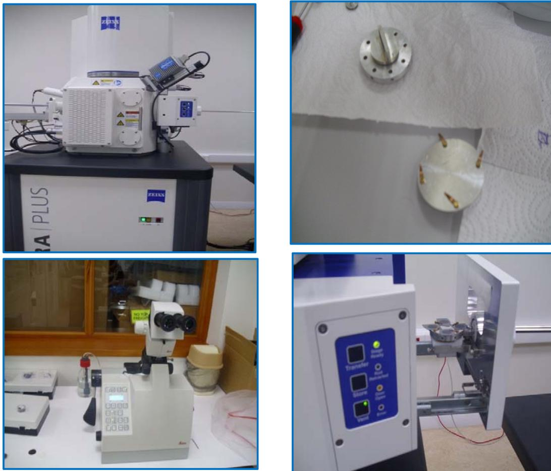
Fig.3. images of instrument (SEM), samples input instrument of SEM, holders of samples (top-view) and (cross-section) and instrument of polishing
