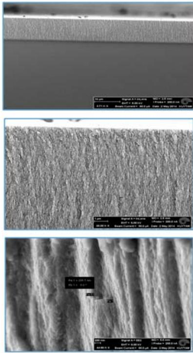
Fig. 5. SEM image (cross-section) of porous silicon sample prepared by etching time 10 min (after polishing) at magnification (a)3710x, (b) 200x (c) 44670x.
