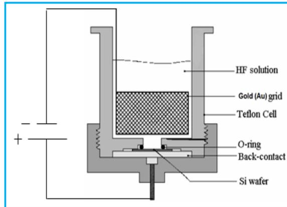
Fig.1. Image of the electrochemical etching set up & Schematic diagram of anodization cell
