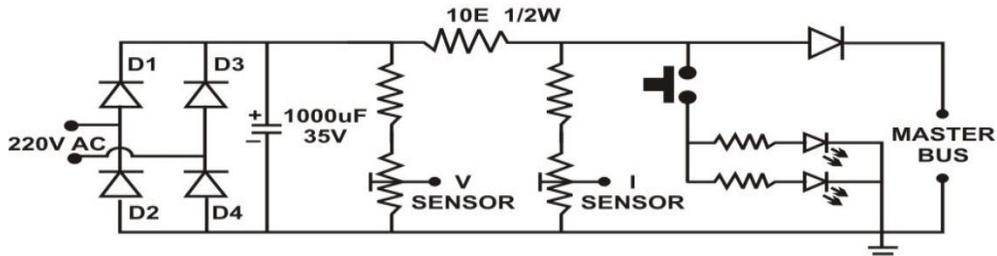
Fig.4 AC Sensing Card for Super Thermal & Nuclear Section
