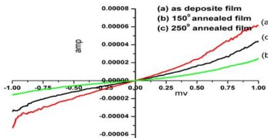
Fig.3 IV measurements of  $\text{CuIn}_3\text{Se}_5$  used for electrical analysis (a)as-deposit film (b)150° C (c)250° C annealed film
